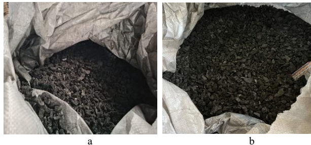
Fig. 1 The produced batches of high-resistivity coke (a) and high-temperature coke (b)
