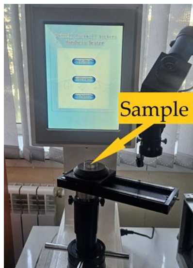
Fig. 3 Hardness measurement process of samples using the THBRV-187.5DX hardness testing device.
