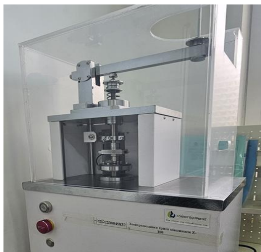
Fig. 4 Hengxu MPX-3 device for determining wear resistance.
