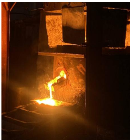
Fig. 3 Tapping of manganese ligature from the ore-thermal furnace during pilot-scale experiments
