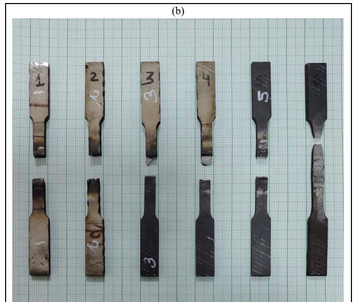
Fig. 3: Tensile test specimens: (a) Before the test; (b) After the test
