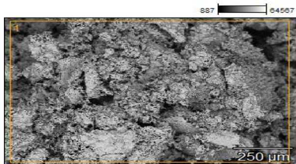
Fig. 3 Iron sponge after hydrogen reduction (two independent runs)
