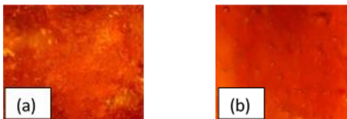
Fig. 4 Structure of the mixture: a – constant pressure; b – variable pressure (×500)
