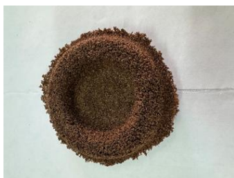
Fig. 13 – Shell mold: with 4% white spirit content
