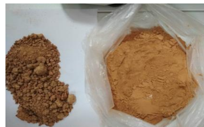
Fig.4 – Fine and large chamotte fractions
