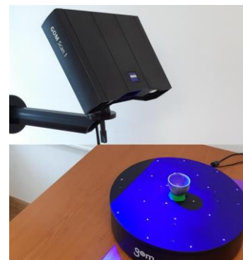
Fig. 4 Photogrammetric system GOM Scan 1 MV400
