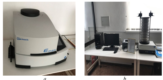
Fig.2 Equipment used for the preparation of inoculators: a – Emax mill; b – Retch analytical screening machine
