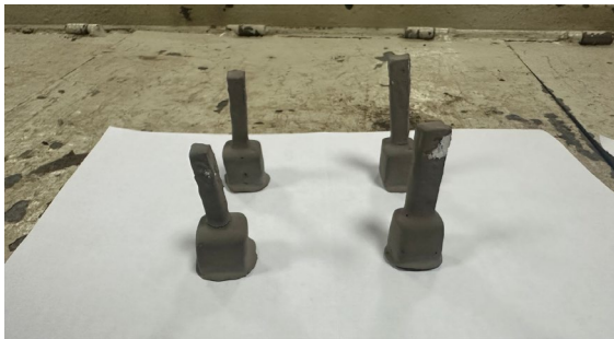
Fig. 3 Ready-made samples for casting
