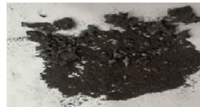
Fig.1 Metal droplets extracted from slag used for inoculators
