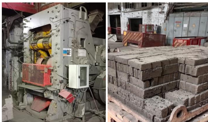
Fig. 1 Semi-dry hydraulic press and CRP briquettes
