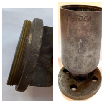
Fig. 2 Capsule for the calcination of ammonium metavanadate (AMV)
