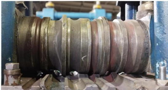
Fig. 7 Design of the roll with combined classical and inclined oval passes (a) and installation of the roll in the laboratory stand (b)
